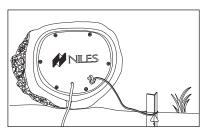
Figure 13 Security Stake Driven into Ground
